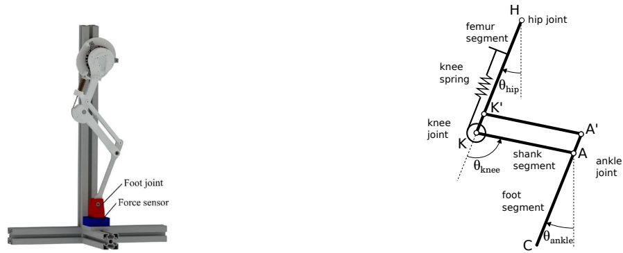
(a) Rendered leg test stand with leg fixed into a rotary joint on hip and foot (red) on force sensor (blue). (b) Schematic of cheetah-cub's spring-loaded leg mechanism.
